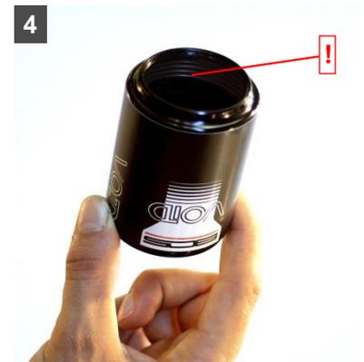
Note your shock pressure, taking into account the loss of pressure when connecting your pump. Slowly deflate the shock. The shock body will retract slightly.
