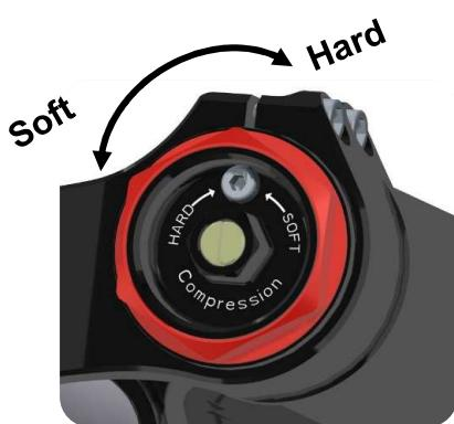
Adjust the compression damping using the flat screwdriver by acting on the compression screw in the center of the top cartridge cap.
