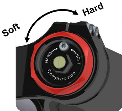
Adjust the compression damping using the flat screwdriver by acting on the compression screw in the center of the top cartridge cap.
