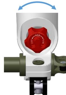
**Compression adjustment** is done by the position of the red lever at the top of the right fork leg. This lever has three positions. The total possible lever movement is 180°; however, the start position may be offset by an angle of about 20° from vertical, as shown in Figure 1.
