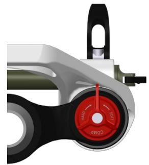
**The three positions** are identified as S (soft), M (medium), and H (hard). The two extremes, S and H are reached at the fully open and fully closed positions of the lever. The M position is the click when moving between the S and H position, for fast and intuitive adjustment on the fly.
