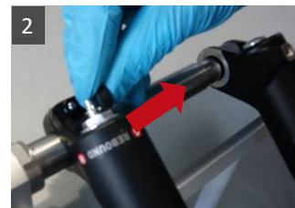
14 Loosen the oil cartridge nut.
