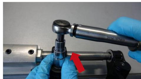
15 Disassemble the oil cartridge from the chassis
