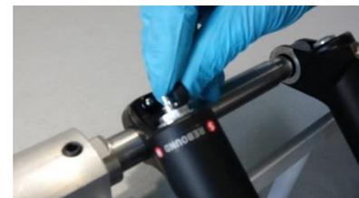
21 Put complete oil cartridge inside the casting.
