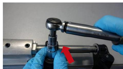
15 Disassemble the oil cartridge from the chassis
