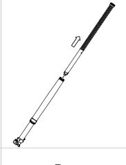
• Carefully remove the spring cartridge from the fork tube
