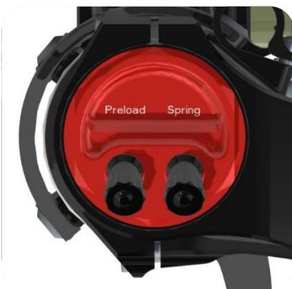
The air pressure is adjusted by the « SPRING » valve.
