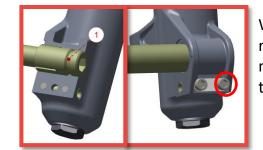
When removing 15 mm x 110 mm axles, make sure not to loosen the right screw (circled in red in the image) to prevent the insert (1) from moving. This precaution does not apply to 20 mm x 110 mm axles. The tightening torque for each screw is 4 Nm.
