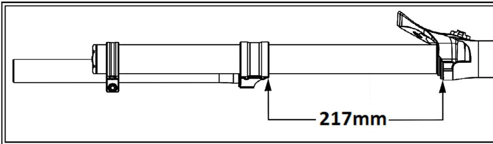
Measure the distance from the top of the leg (lower part of the seal) to the bottom of the lower crown
