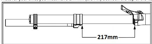
Measure the distance from the top of the leg (lower part of the seal) to the bottom of the lower crown
