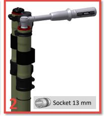
2 Once the pressure is released, use a 13 mm socket to unscrew the black cap located at the top of the stanchion.
