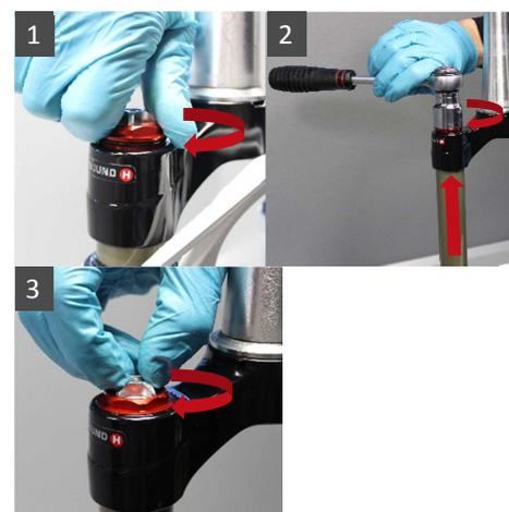
*No torque – tighten to contact*
