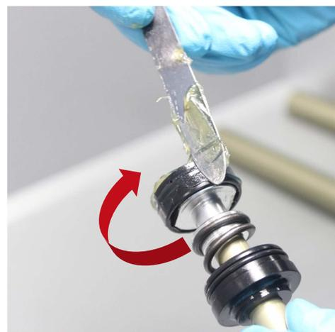
*The groove should be full of grease!*
