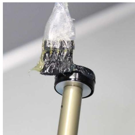
*The groove should be full of grease!*
