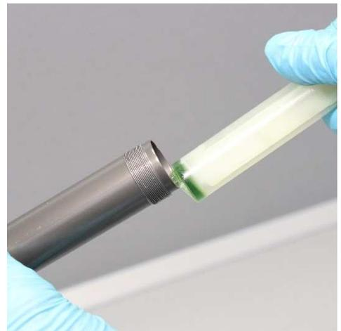
**33 Shaft guide screwed on the cartridge**
