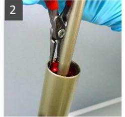
**32 Shaft guide screwed on the cartridge (skip to step 36 if shaft guide clamped)**
