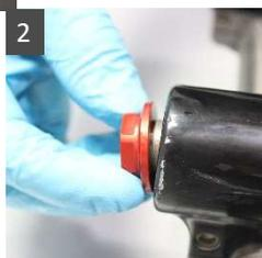
**6** Screw the oil cartridge cap on the first threads by hand.
